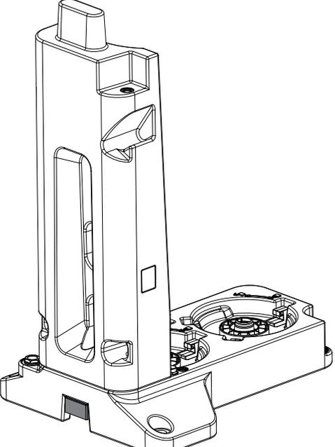
A technical line drawing of the same vertical device as in the previous image. The locking device is now fully inserted into the slot at the bottom, and the arrow is no longer present.                                                                                                | <p>13. Press the locking device into the locking device opening as far as it will go.</p>                                          |
