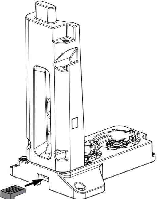
A technical line drawing of a vertical, rectangular device with a handle on the left and a circular opening on the right. A small, rectangular locking device is shown being inserted into a slot at the bottom of the device. An arrow points from the locking device towards the slot. | <p>12. Align the locking device with the heel facing downwards and insert it into the locking device opening in the collector.</p> |
