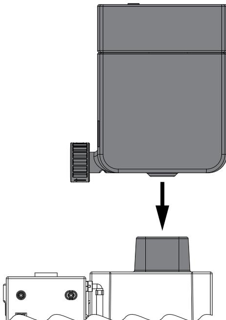
17. Place the pressure relief chamber on the foot.
