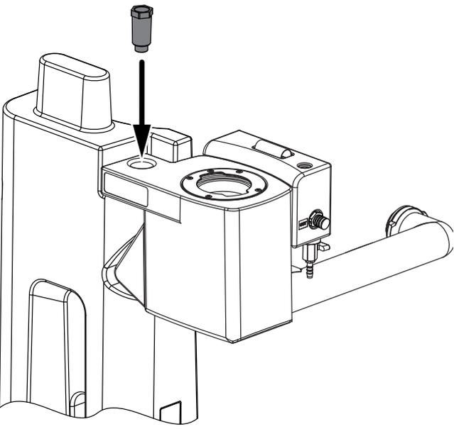
A technical line drawing showing the measuring chamber now seated in the holder. A grey screw is shown above the chamber with an arrow pointing down into a hole on its top surface.                           | 15. Insert the fixing screw into the fixing hole of the measuring chamber. |
