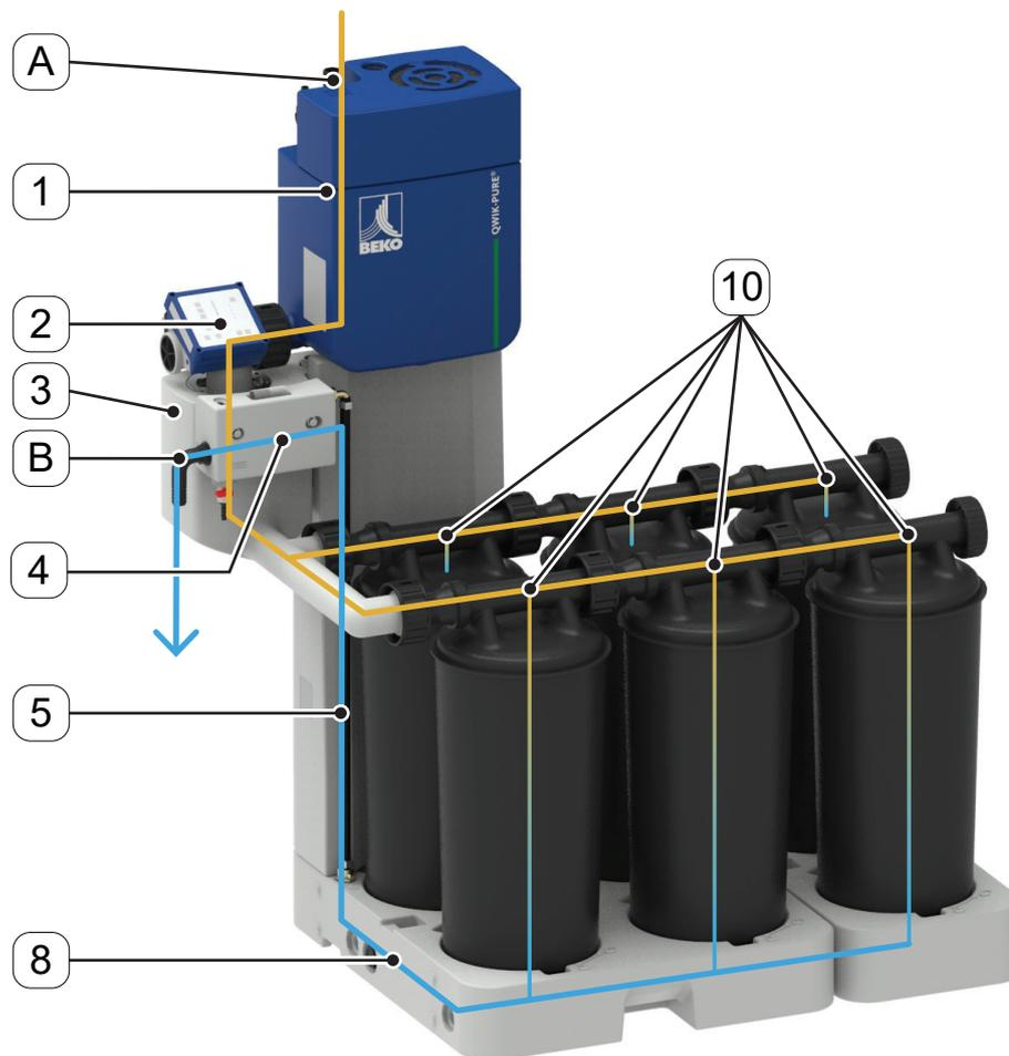
The condensate is fed from the condensate collection line via the condensate inlet **[A]** into the pressure relief chamber **[1]**. In the pressure relief chamber **[1]**, entrained compressed air is separated before the condensate flows through the **FRC [2]** into the measuring chamber **[3]** and then into the filter cartridges **[10]**.
