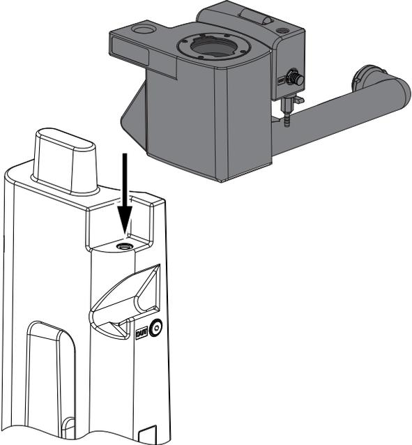
A technical line drawing showing a grey measuring chamber being lowered into a white holder. The holder is mounted on a vertical post. An arrow points downwards from the chamber towards the holder's opening. | 14. Insert the measuring chamber into the holder in the foot.              |
