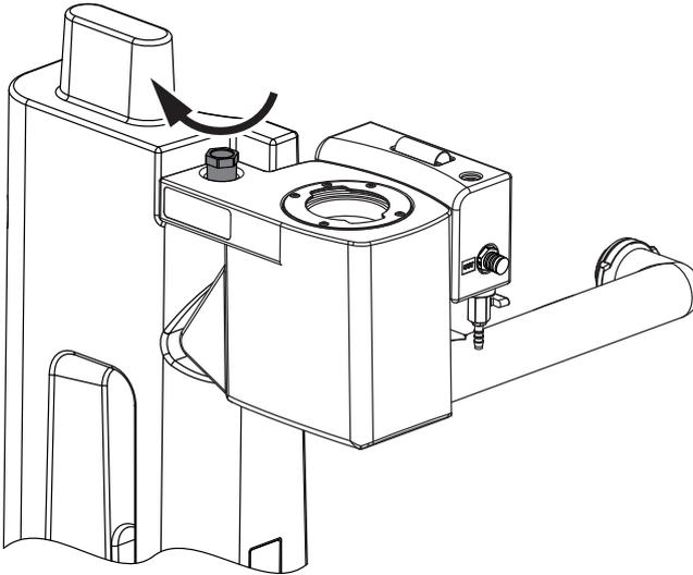
16. Screw in the fixing screw clockwise by hand all the way and tighten hand-tight.
